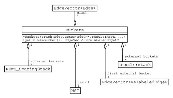
Figure 4.4: UML class diagram - node reduction with buckets
