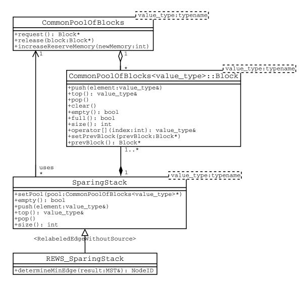
Figure 4.3: UML class diagram — internal buckets
