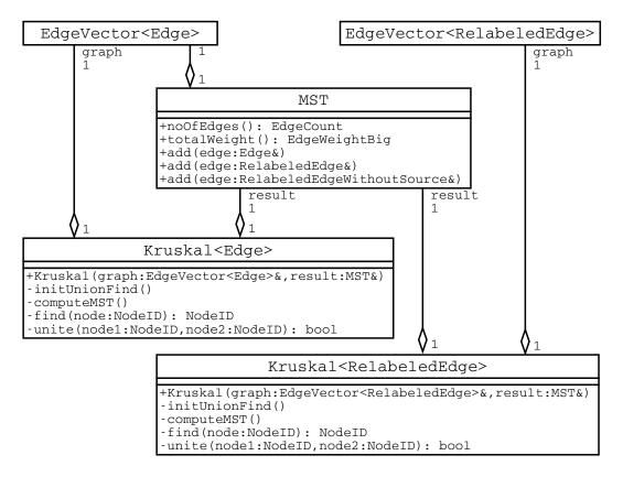
Figure 4.2: UML class diagram — Kruskal's algorithm
